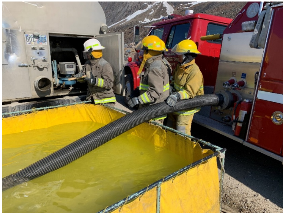
Pictured Above: A Fire Department Training Officer demonstrating drafting techniques to effectively supply the fire truck with water
